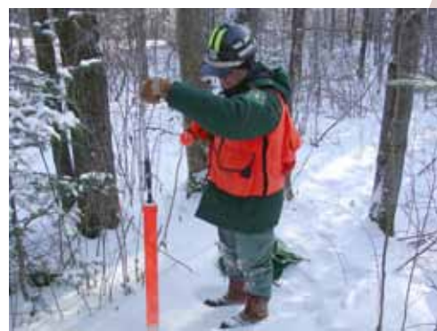
Frost tubes are easily installed at a unit and help determine the depth of frozen ground.
